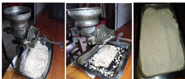
Figure 2. Representative image of milling and obtaining flour from Phaseolus Vulgaris , L.
