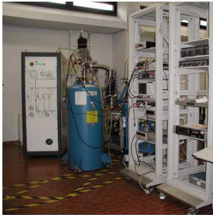
Figure 3.4. The entire experimental setup composed by the dilution refrigerator inside the dewar with the Gas Handling System (GHS) for the injection of the ^3\text{He} - ^4\text{He} mixture.
