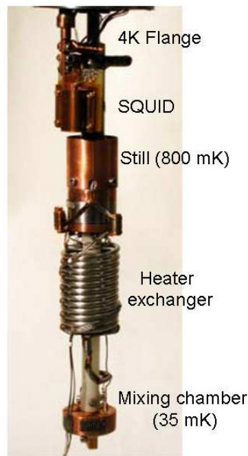
Figure 3.3. Dilution refrigerator composed by the 4K stage, where the SQUID is mounted, the still at 800 mK, the heat exchanger and the mixing chamber.
