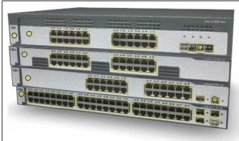
Figura 4-7: Vista frontal de Switch Cisco 3750.
