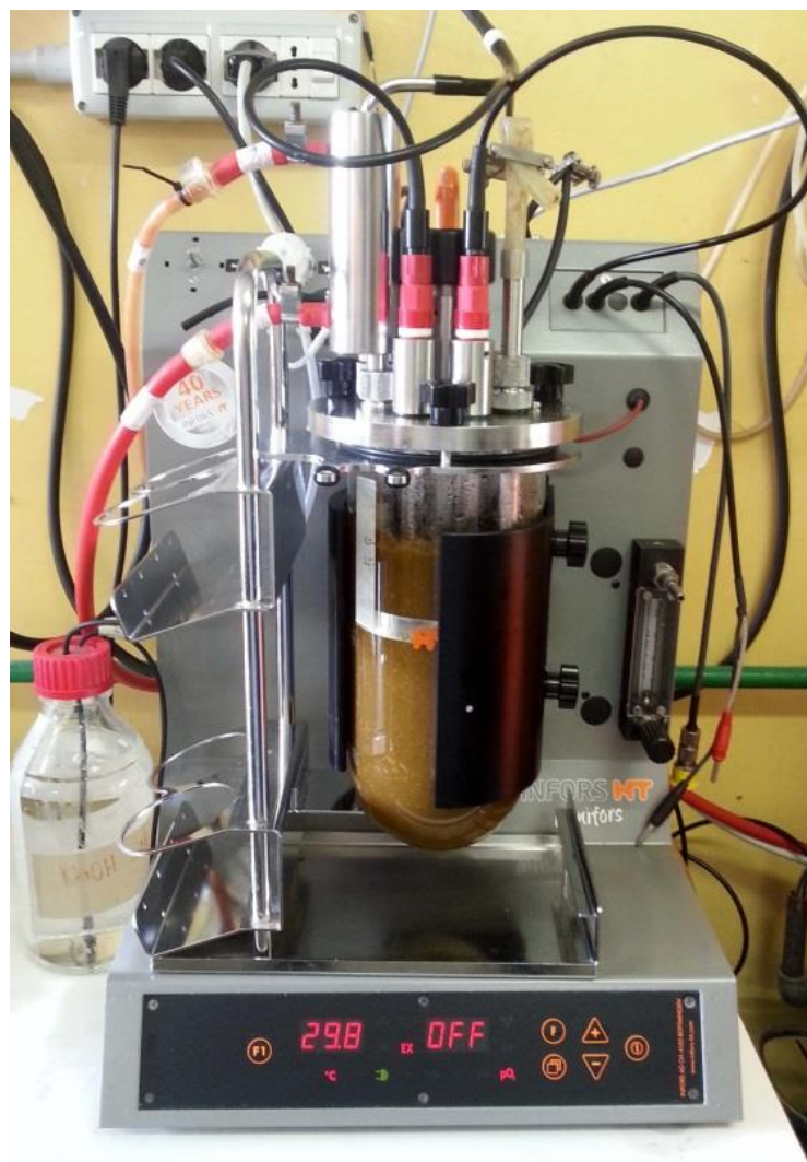
Figure 12. "MINIFORS INFORS" reactor
