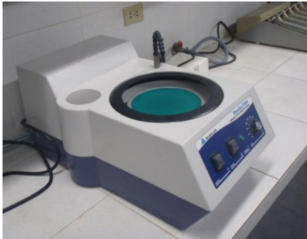
Fig. 17 Pulidora Metaserv 3000 variable speed grinder-polisher marca Buehler
