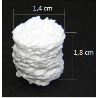
Figure 5. Photographs of \gamma -alumina foams prepared from polyurethane “C” and synthesized \gamma -alumina.
