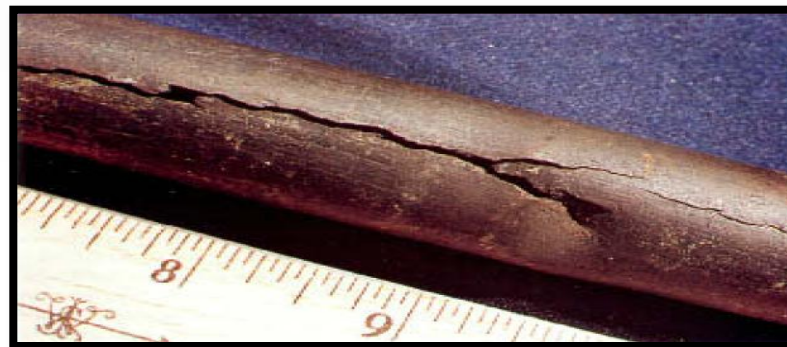
SCC(Stress Corrosion Cracking)
