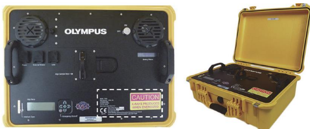
Fig I. Olympus Terra Portable X-Ray Diffraction/Fluorescence instrument
