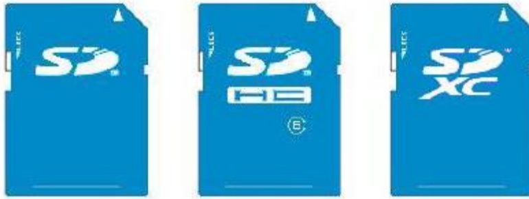
Figura 26: Memorias SD, SDHC y SDXC [19]
