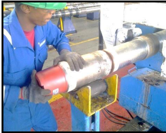
Figura 3. 43: Instalacion de Crossover [17]
