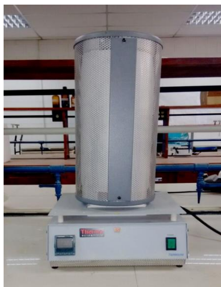
Figura N° 2. Horno tubular modelo THERMOLYNE TUBE FURNANCE F21135
