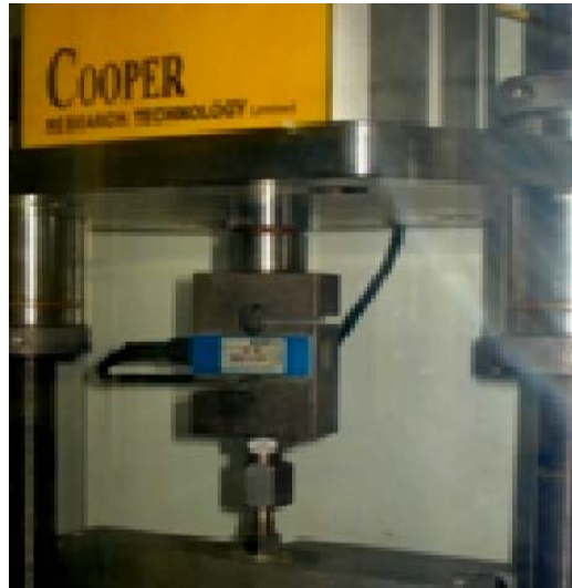
Figure 4.31: Screw bolt connection between load frame and loading cell
