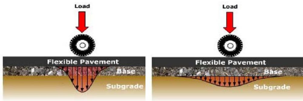
Figure 1.8: Flexible Pavement Load distribution (WAPA)
