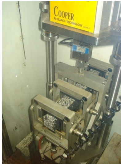
Figure 4.29: NAT during a four-point bending fatigue test
