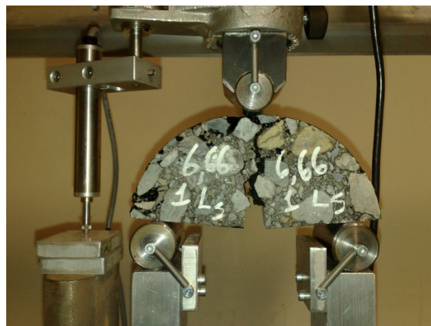
Figure 4.20: Failure of Specimen during SCB Test
