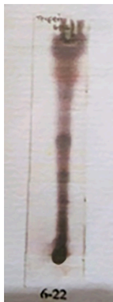
Figure 2. Stain Appearance: Sulfuric Acid Anisaldehyde Reactor.
