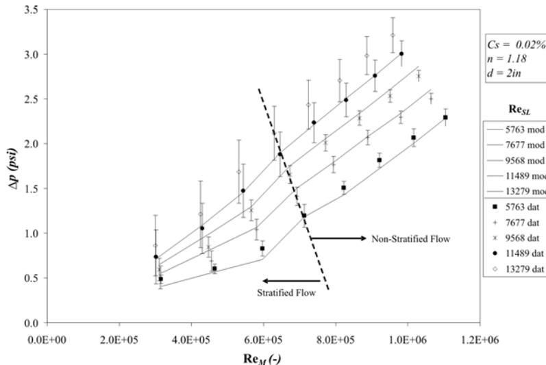
**Figure 7.** Pressure Drop vs. Mixture Reynolds Number ( $C_S = 0.02\%$ ,  $n = 1.18$ ,  $d = 2$  in.).
