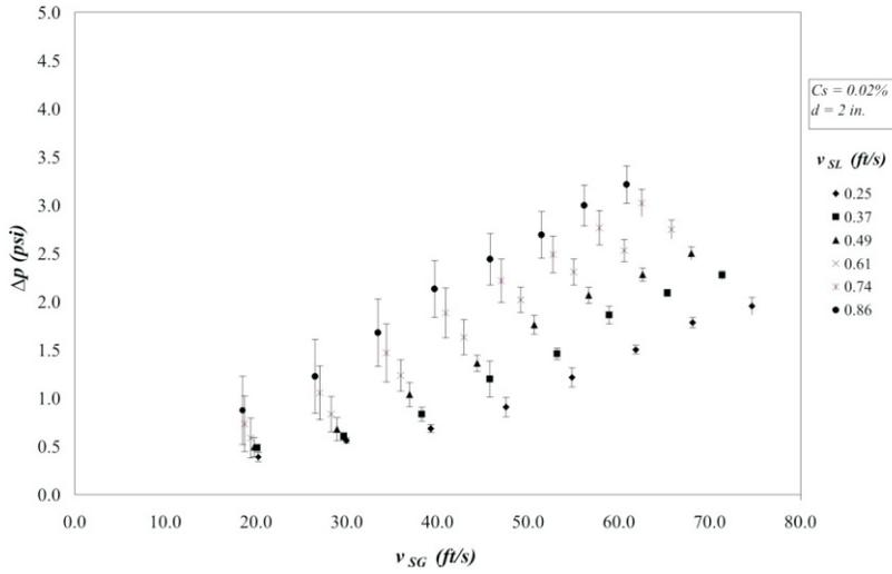
**Figure 4.** Foam Flow Pressure Drop vs. Gas Flow Rate Results ( $C_s = 0.02\%$ ,  $d = 2$  in.).
