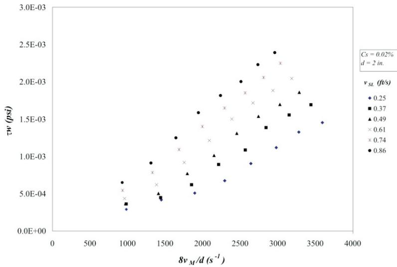
**Figure 5.** Foam Flow Wall Shear Stress vs. Shear Rate Results ( $C_s = 0.02\%$ ,  $d = 2$  in.).
