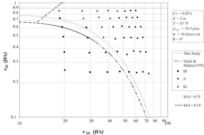
**Figure 8.** Comparison of Prediction of Flow Pattern Maps for Foam Flow ( $C_s = 0.02\%$ ,  $T = 85^\circ\text{F}$ ).
