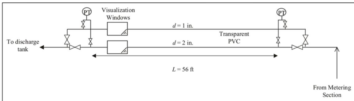
**Figure 1.** Schematic of Rheology Section.
