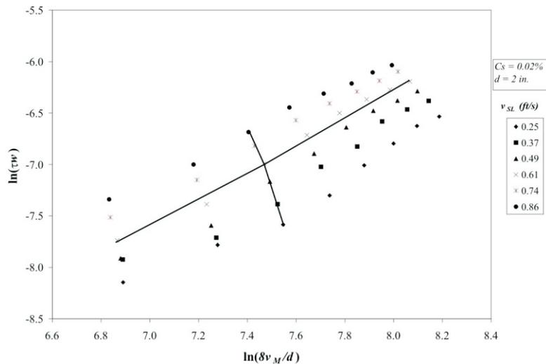
**Figure 6.** Foam Flow Wall Shear Stress vs. Shear Rate Results in Logarithmic Scale ( $C_s = 0.02\%$ ,  $d = 2$  in.).
