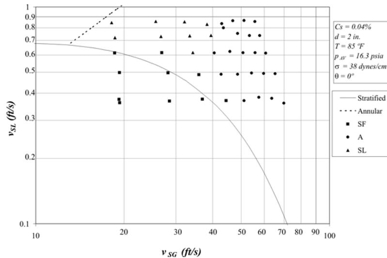
**Figure 3.** Foam Flow Pattern Results in 2 in. Diameter Rheology Pipe Section for  $C_s = 0.04\%$  Plotted on Taitel and Dukler (1976) Map.
