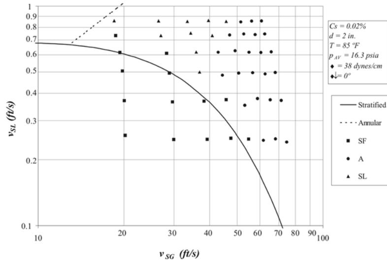
**Figure 2.** Foam Flow Pattern Results in 2 in. Diameter Rheology Pipe Section for  $C_s = 0.02\%$  Plotted on Taitel and Dukler(1976) Map.
