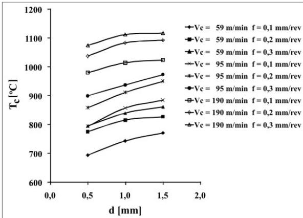
**Figure 4.** Cutting temperature vs. depth of cut for AISI 304 stainless steel
