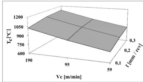
**Figure 9.** Cutting temperature vs. cutting speed and feed, when turning AISI 304 steel with a depth of cut of 1,5mm
