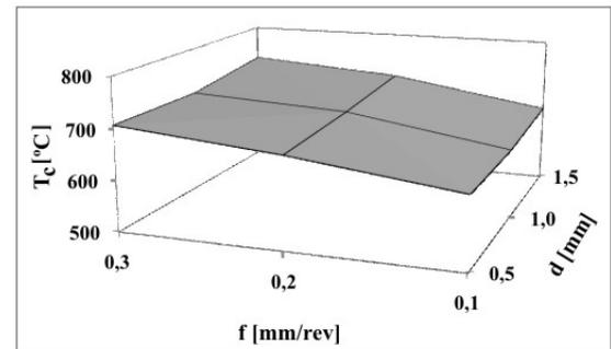
**Figure 17.** Cutting temperature vs. feed and depth of cut, when turning AISI 420 steel at a cutting speed of 190 m/min
