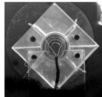
**Figure 2.** Scheme of the four coils distributed around the lathe rotary axis
