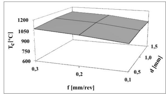
**Figure 15.** Cutting temperature vs. feed and depth of cut, when turning AISI 304 steel at a cutting speed of 190 m/min
