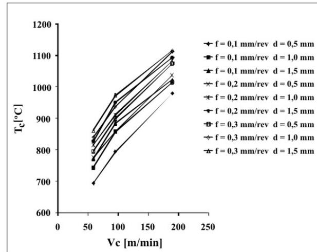
**Figure 6.** Cutting temperature vs. cutting speed for AISI 304 steel
