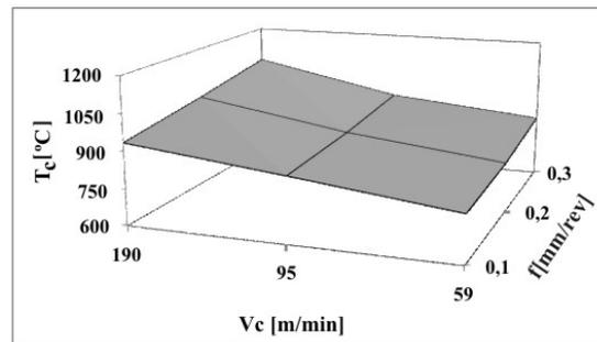
**Figure 10.** Cutting temperature vs. cutting speed and feed, when turning AISI 316L steel with a depth of cut of 1,5mm
