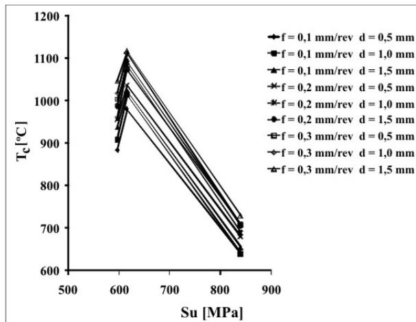
**Figure 8.** Cutting temperature vs. maximum strength when using a cutting speed of 190 m/min
