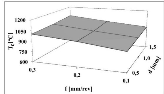
**Figure 16.** Cutting temperature vs. feed and depth of cut, when turning AISI 316L steel at a cutting speed of 190 m/min
