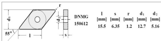
**Figure 1.** Scheme of the tip geometry used in the experiment
