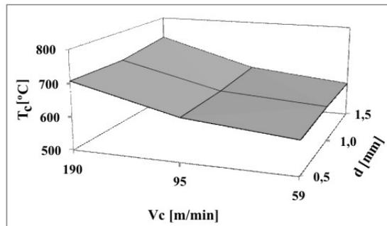
**Figure 14.** Cutting temperature vs. cutting speed and depth of cut, when turning AISI 420 steel with 0.3 mm/rev
