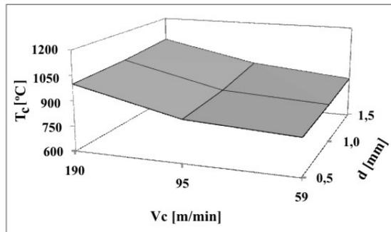
**Figure 13.** Cutting temperature vs. cutting speed and depth of cut, when turning AISI 316L steel with 0.3 mm/rev
