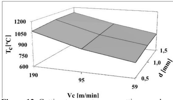
**Figure 12.** Cutting temperature vs. cutting speed and depth of cut, when turning AISI 304 steel with 0.3 mm/rev
