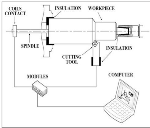
**Figure 3.** Scheme of the experimental tool-work thermocouple arrangement for cutting temperature measurement
