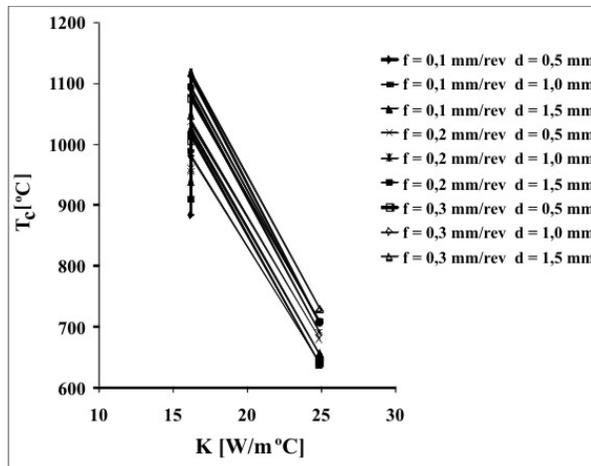
**Figure 7.** Cutting temperature vs. thermal conductivity when using a cutting speed of 190 m/min
