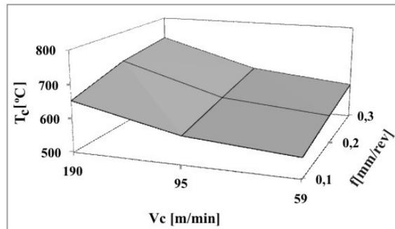
**Figure 11.** Cutting temperature vs. cutting speed and feed, when turning AISI 420 steel with a depth of cut of 1,5mm
