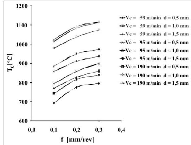
**Figure 5.** Cutting temperature vs. feed for AISI 304 steel
