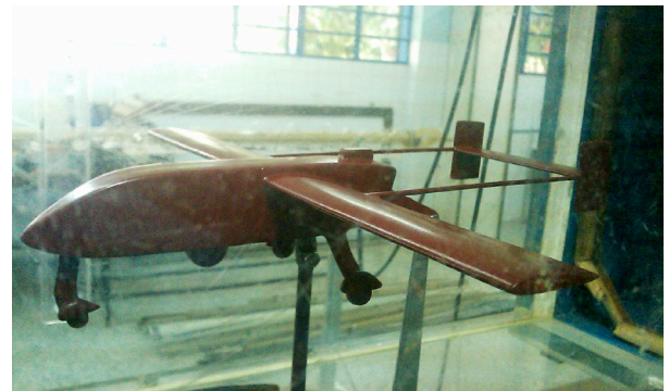
Figure 7. Modified airplane (ANCE X-3) model in the wind tunnel
