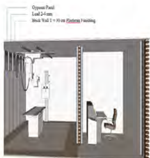
Figure 4 Details of Lead Application in X-Ray Room
