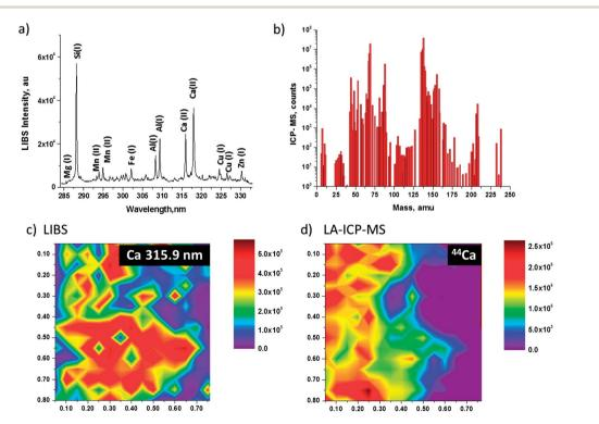
Fig. 2 Representative LIBS (a) and LA-ICP-MS (b) spectra acquired from a single location of the sample. (c and d) Surface (2D) distribution of Ca of the same  $0.785 \times 0.785$  mm<sup>2</sup> area of a *Bastnäsite* rock sample. The Ca maps were obtained simultaneously by (c) LIBS and (d) LA-ICP-MS.
