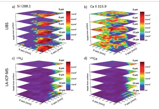
Fig. 4 Layer-by-layer contour elemental maps obtained by simultaneous LIBS/LA-ICP-MS. (a and b) LIBS and (c-d) LA-ICP-MS maps as a function of depth.
