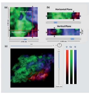
Fig. 5 Merged overlay of U, Ca and Si maps. (a) 2D layer imaging, (b) 2D cross-sectional imaging and (c) 3D reconstruction of the elemental distribution in the *Bastnäsite* rock matrix. All data are plotted using a linear color scale where the brightest colors represent the highest intensity. Lateral scale:  $0.785 \times 0.785$  mm<sup>2</sup>, axial scale: 15  $\mu$ m.
