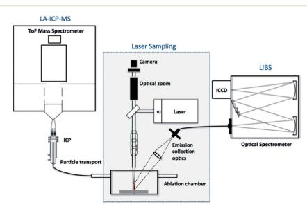
Fig. 1 Experimental setup for simultaneous LIBS and LA-ICP-MS.
