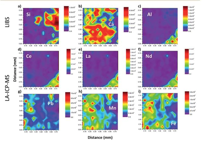
Fig. 3 Simultaneously obtained 2D LIBS surface maps of the *Bastnäsite* rock sample using LIBS and LA-ICP-MS. (a–c) LIBS elemental maps of Si I (288.1 nm), Ca II (315.9 nm) and Al I (308.2 nm). (d–i) LA-ICP-MS maps of <sup>140</sup>Ce, <sup>139</sup>La, <sup>146</sup>Nd, <sup>208</sup>Pb, <sup>55</sup>Mn and <sup>57</sup>Fe.
