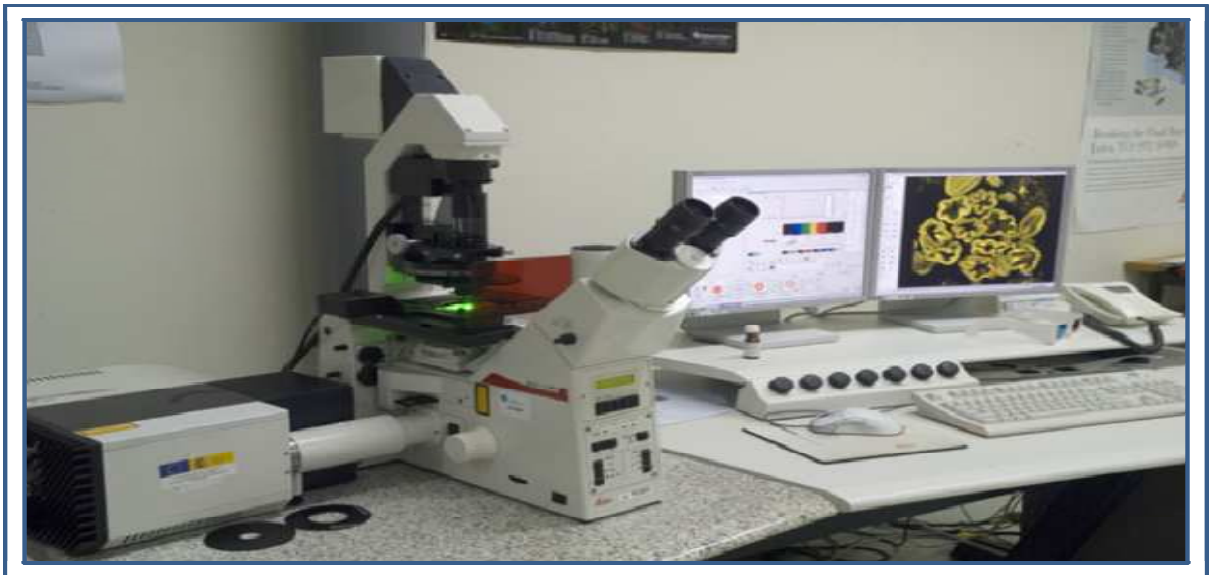
Figura 28. Imagen del Microscopio Láser Confocal Leica TCS SP2 AOBS. Rapid Scanning Confocal Microscopy. Cell Biological Applications of Confocal Microscopy. Edited by M. Matsumoto. Fuente: www.vet.unicen.edu.ar/..Microscopia%20de%20laser%20confocal%20PDF.pdf . 2006.
