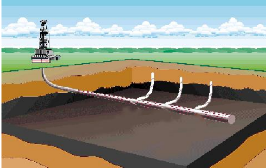
Figura 2.9 Pozo multilateral “Backbone and Rib” . Fuente (9)
