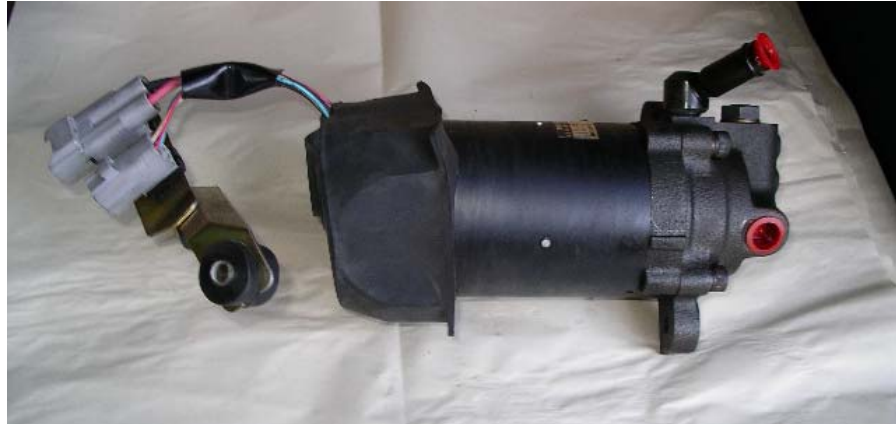
Figura 63. Bomba Electro-hidráulica de Toyota MR2. Tomado de Other Systems: Power Steering por Cameron Motor Works Electric Vehicle Conversion (2005).
