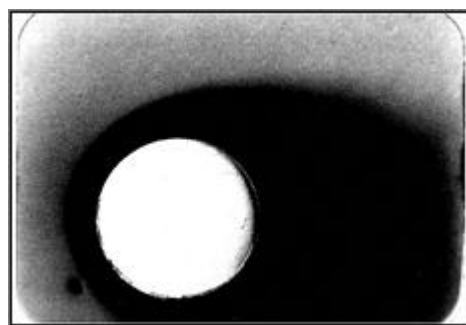
Figure 6. Image of an X-Ray film exposed to the collimated \gamma radiation, with a 25 mm diameter sample superimposed on it
