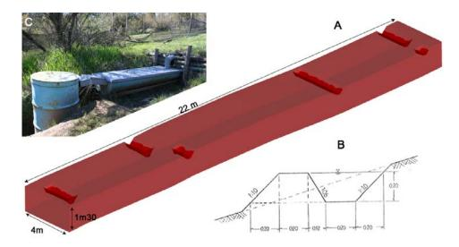
**Figure 2.** (a) Layout of the infiltration trenches on the Wishmeier plot, (b) trench dimensions and (c) collector drums at the plot outlet.
