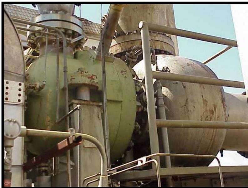
Figura 5. 18: Expansor/ precompresor <sup>[28]</sup>
