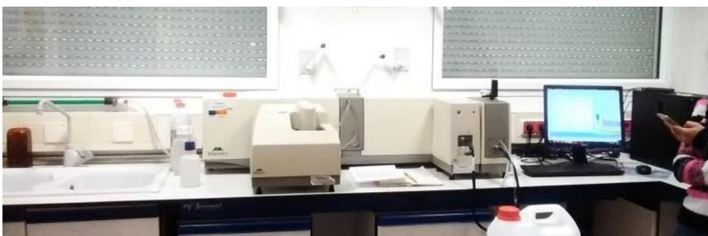
Figura 6. Master Sizer 2000LF de Malvern Instruments.
