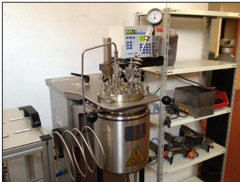
Figura 3.8 Detalle del reactor autoclave (Büschiglassuster stirrer vessel type 3)
