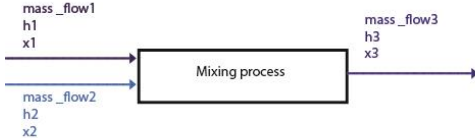
Figure 5 – Schematic mixing process
