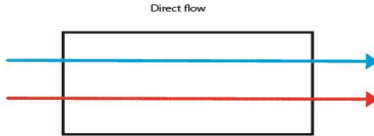
Figure 35 – Direct flow heat exchanger
