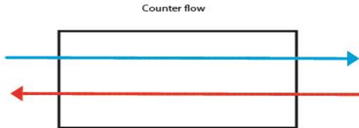
Figure 36 – Counter flow heat exchanger
