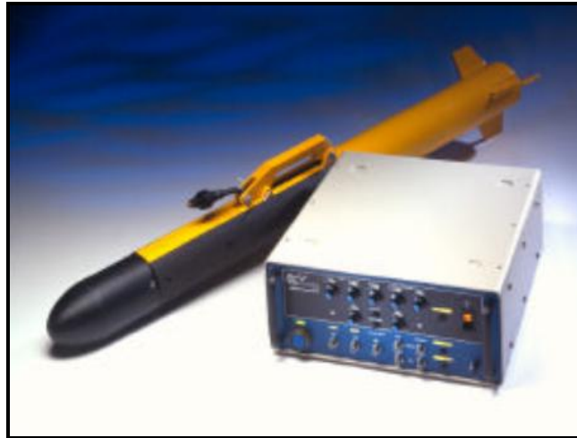
Figura 2.4 Sonar de Barrido Lateral ( Side Scan Sonar ) GeoAcoustics
