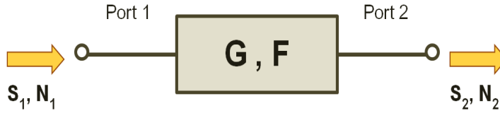
Figure 4.1.4: Schematic representation of a 2-port network.
