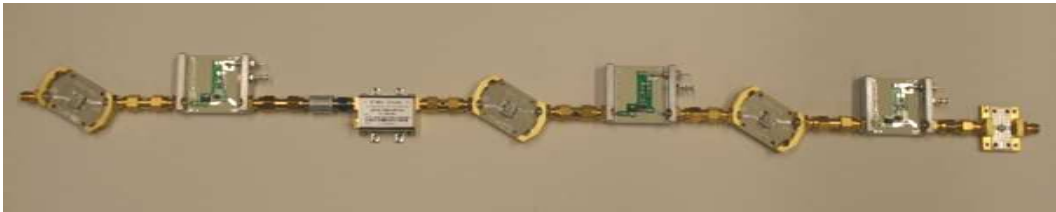
Figure 7.2.4: Photograph of the RF reception path built with the selected COTS components.
