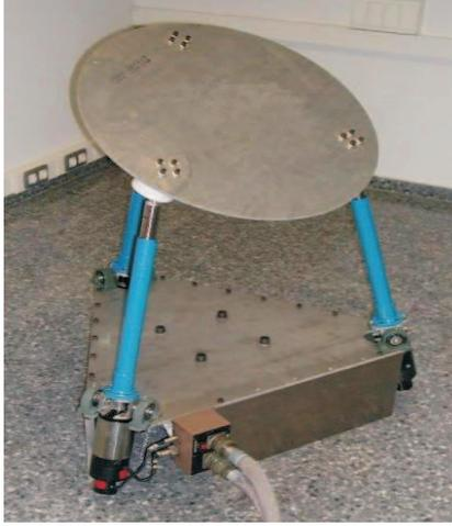
Figure 1: Actual 3-RPS parallel robot
